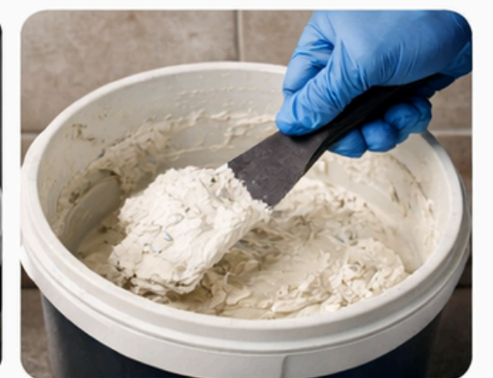
Close-up view of ready-to-use epoxy grout with smooth consistency.
